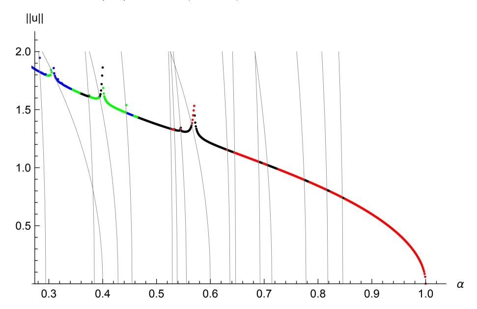
The nonlinear wave equation, truncated at  $N \gg K = 7$ . The (1,1) branch undergoes a <u>fold</u> bifurcation at  $\alpha \simeq 0.571$ and a <u>pitchfork</u> bifurcation involving the (5,3) branch at  $\alpha \simeq 0.585$ .
